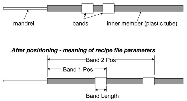
After positioning each band, the machine uses Blockwise's 6-jaw precrimper to form the band into a hexagonal shape that holds it firmly in position for swaging.
