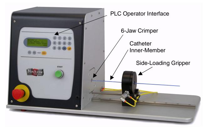
The band positioner / precrimper model PMC uses a simple, reliable, mechanical approach to positioning bands, with no optical sensors or vision systems. The PLC control software can be set up by a novice in just a few minutes.
