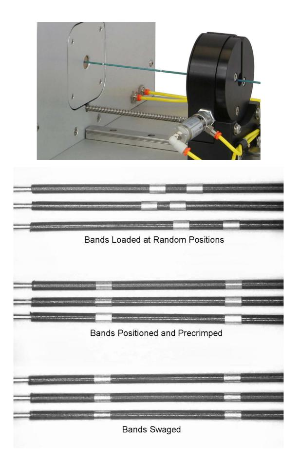
Cycle time depends on the process settings; typical cycle time for PTCA-type catheters is about 28 seconds.
